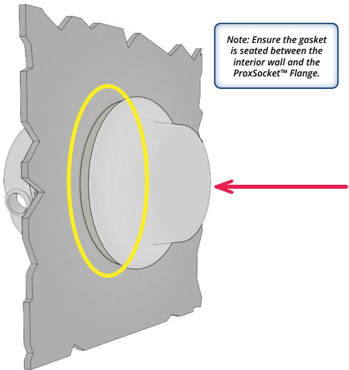
*Note: Ensure the gasket is seated between the interior wall and the ProxSocket™ Flange.*
