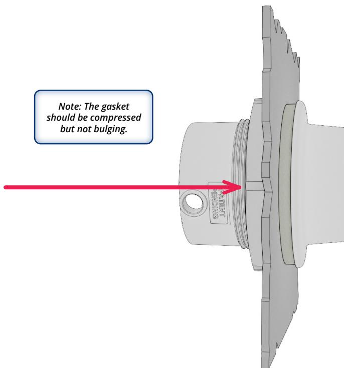
4. Hand tighten the sensor into ProxSocket™ body until it reaches the inside face
